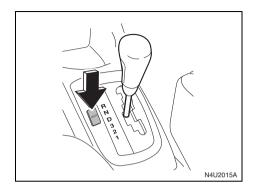
Press the HOLD button on the shift lever to turn on the HOLD mode.
